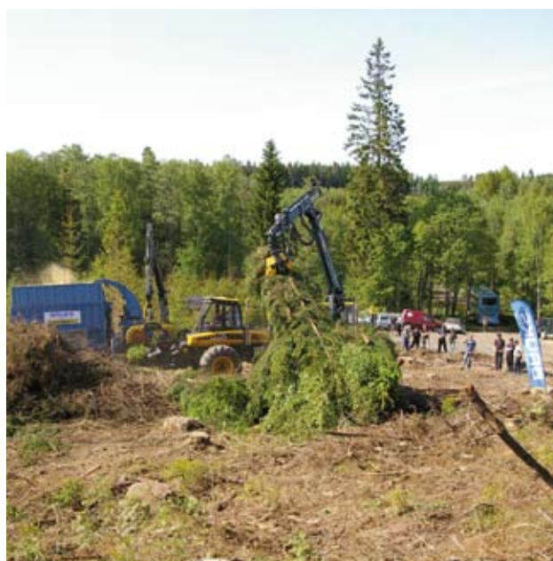
Harvesting and chipping of logging residues.
